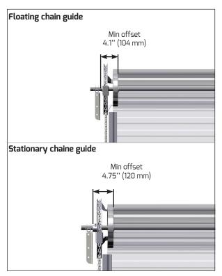
Chain hoist may be mounted on either side of the door.
